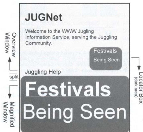
FIGURE 5. Magnifier-plus-overview mode in Experiment 2. Magnified window (bottom) and the overview window (top) are displayed on the same screen.
